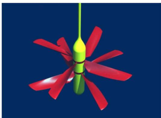
Fig. 11. Turbine with double counter-rotating rotors (red) connected to a cable (not shown) and suspended about 100 m below a float.
