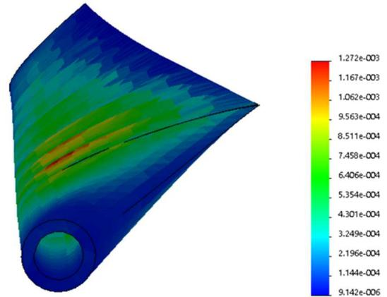
Fig. 8. Strain levels at the surface of the blade. Red are the highest strain levels and blue are the lowest strain levels. The strain values should be multiplied by a factor ten. With 1.27% the highest strain level stays below 2%.
