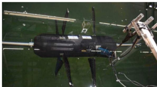
Fig. 12. Scale model test of the Subwave turbine in Stadt Towing Tank, University College of Western Norway.
