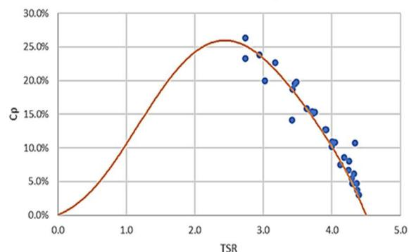
Fig. 13.  $C_p$  versus TSR for the measurements (blue dots) in Stadt Towing Tank, as well as a typical  $C_p$  versus TSR curve (orange) drawn through the measurements for illustration.
