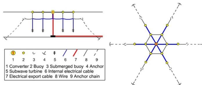
Fig. 15. A park of Subwave turbines suspended from buoys. Six anchors and one tension mooring hold twelve units and a central unit for electrical conversion and export. Profile at left, top view at right.
