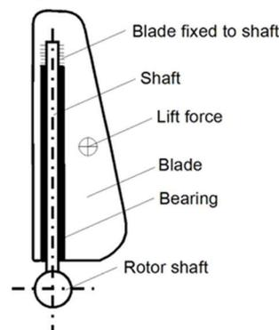
Fig. 1. Schematic cross section of the Waveco tidal blade.
