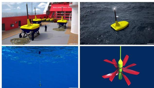
Fig. 16. Self-positioning ocean observation platform (top figures) with the Subwave turbine suspended underneath (lower figures).
