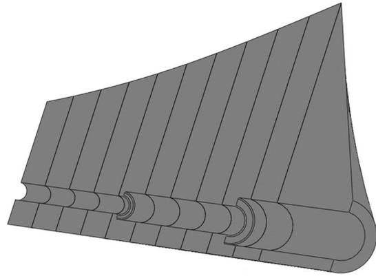
Fig. 5. Cross section of the 3D blade model showing the tapered hole that runs through the blade from the root to the tip.
