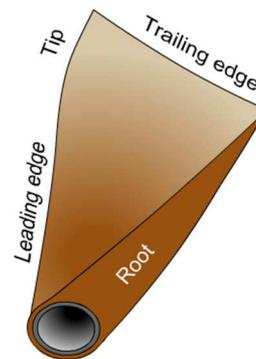
Fig. 2. Simplified 3D drawing of a flexible blade design. We see the blade twist to the right. The blade can also twist to the left.
