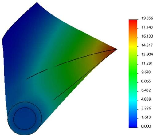
Fig. 7. Deformation (displacement) of the surface of the Waveco blade under loading seen from the root (deformation in mm). The deformation values should be multiplied with a factor of ten.
