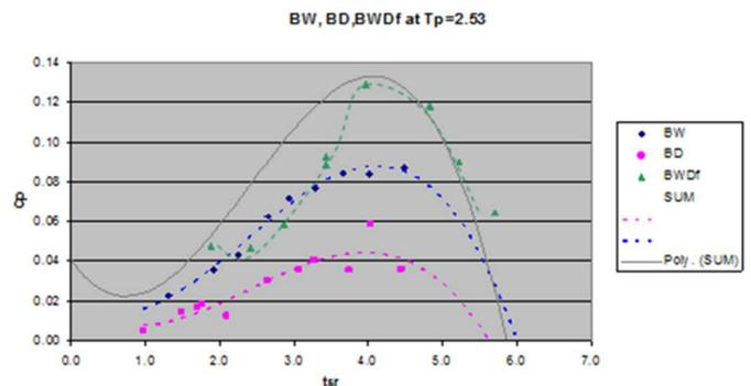
Fig. 10.  $C_p$  versus TSR; scale test results at Ifremer France, for different turbine configurations in regular waves (wave height = 0.4 m, wave period = 2.53 s). BW is only a Wells-rotor, BD is only a Darrieus rotor and BWDf is a combined Wells and Darrieus rotor. Poly (SUM) is the addition of the BW and BD polynomials.
