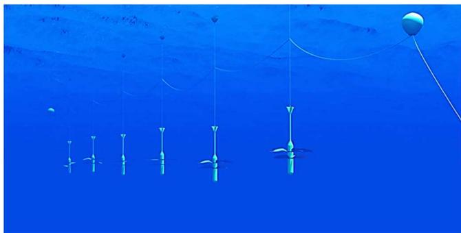
Fig. 14. Several Wavecو's unidirectional counter-rotating double rotor turbines suspended under floating buoys.
